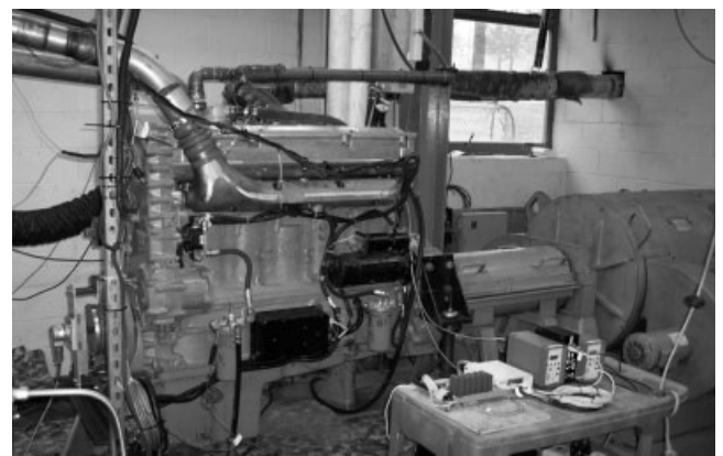
Fig. 1 WVU test cell with 1992 Detroit Diesel Series 60 engine mounted
